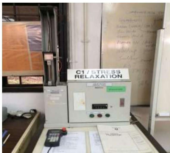
Figure 1. C_1 /Stress relaxation machine
